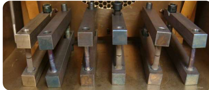
Solid Metal Embrittlement Coupons Mounted in Test Fixtures
